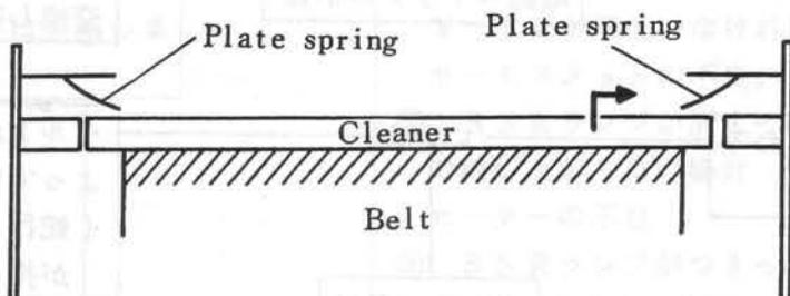
Pull the knob of the SCRAPER STAY attached to the RECEIVER, so that you will find a DRUM CLEANER on the inner part of the RECEIVER.
